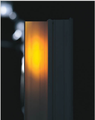
Light penetration of competitor's vinyl material
