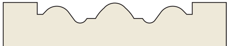
SM-19 Rosette 15/16 \times 3-3/4 \times 3-3/4 Cherry | STAIN GRADE | SM19CH Maple | STAIN GRADE | SM19M Oak, Red | STAIN GRADE | SM19O Pine | STAIN GRADE | SM19
