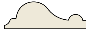
SM-733 1/2 × 1-1/2 Cherry | STAIN GRADE | SM733CH Maple | STAIN GRADE | SM733M Oak, Red | STAIN GRADE | SM733O
