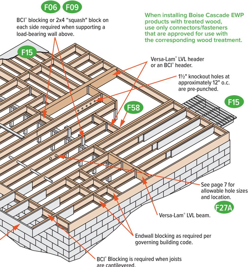
BCI® Joists, Versa-Lam® LVL, and ALLJOIST® must be stored, installed and used in accordance with the Boise Cascade EWP Installation Guide, building codes, and to the extent not inconsistent with the Boise Cascade EWP Installation Guide, usual and customary building practices and standards. Versa-Lam® LVL, ALLJOIST® and BCI® Joists must be wrapped, covered, and stored off of the ground on stickers at all times prior to installation. Versa-Lam® LVL, ALLJOIST® and BCI® Joists are intended
