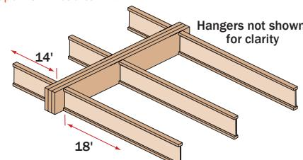
Find: A multiple 1 3/4" ply Versa-Lam® LVL that is adequate to support the design loads and the member's proper connection schedule.
