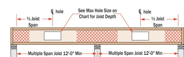
Larger holes may be possible for either Single or Multiple span joists; use BC Calc® sizing software for specific analysis.
