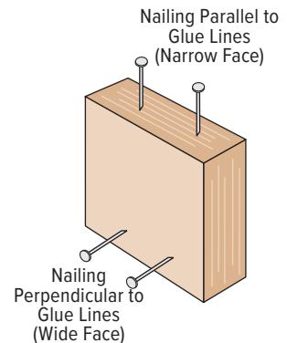
1) For 1¼" thickness and greater, 2 rows of nails (such as for a metal strap) are allowed (use ½" minimum offset between rows and stagger nails).
