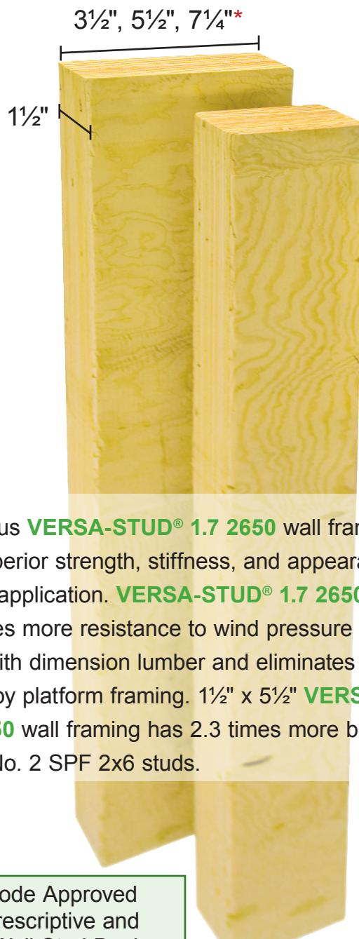
Long, continuous **VERSA-STUD® 1.7 2650** wall framing will provide superior strength, stiffness, and appearance in any tall wall application. **VERSA-STUD® 1.7 2650** wall framing provides more resistance to wind pressure than walls framed with dimension lumber and eliminates the hinge created by platform framing. 1½" x 5½" **VERSA-STUD® 1.7 2650** wall framing has 2.3 times more bending strength than No. 2 SPF 2x6 studs.
