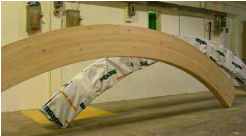
Finished Curved Beams
