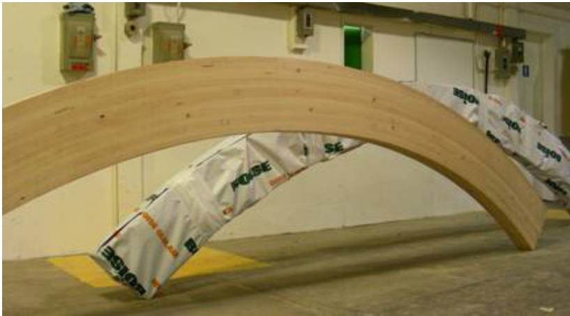
Finished Curved Beams
