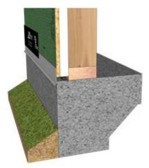
Scenario 3: OSB flush with foundation. Min. 1/2" gap between OSB and foundation.
