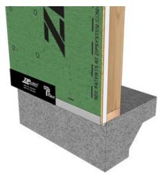
Scenario 3: Drip edge bent to Cover the bottom of the panel.
