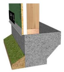
Scenario 4: OSB/foam connection flush with foundation. Min. 1/2" gap between OSB and foundation.
