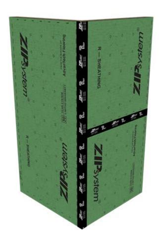
**PRO TIP**: Avoid creating cold corners and nailing voids by shifting over one of the outside corner panels the thickness of the ZIP System® R-sheathing used.
