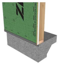
Scenario 4: fluid applied flashing or peel-n-stick membrane along bottom edge of panel onto the foundation.
