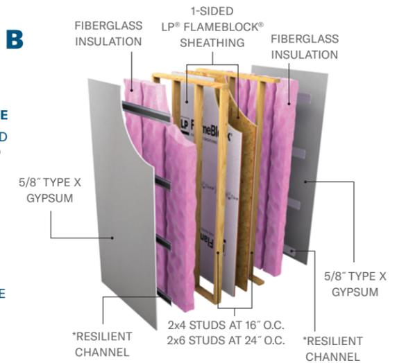
TWO 1-HOUR FIRE-RESISTANCE RATED WALL ASSEMBLIES: IRC SECTION R302.2.1 DOUBLE WALLS
