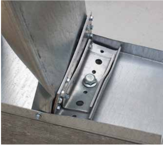
RCKW assembly test with member failure.
