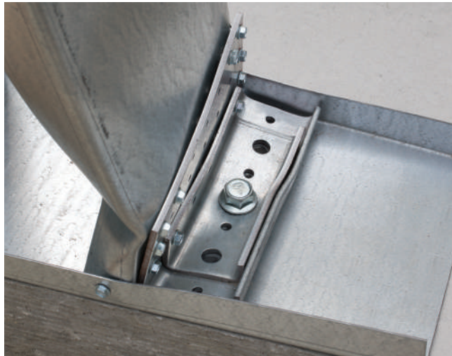
RCKW assembly test with member failure.
