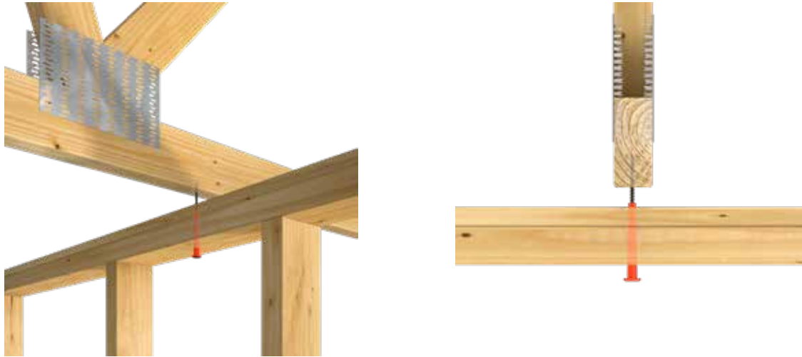
Typical Installation of SDPW DEFLECTOR Screws
