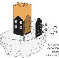
APB88 with optional decorative side plate (Shown using (2) Stainless-Steel Titen HD screw anchors)
