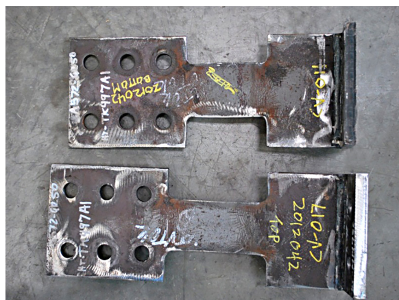
Figure D3.3 — Yielding in Strong Frame Yield-Links
