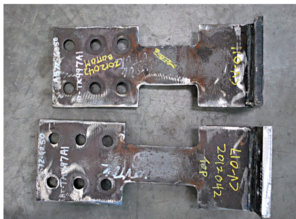
Sample Yield-Link Compression and Elongation from Testing
