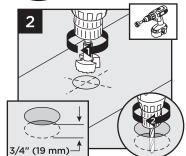
diameter hole in base of the first hole through deck board.
