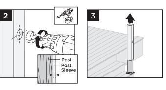
2. Drill a 1" (25 mm) hole through post sleeve. Drill deep enough to mark location on pressure-treated post. 3. Remove the post sleeve from the post.
