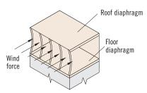
Wind force on a wall is resisted by wall sheathing and framing.
