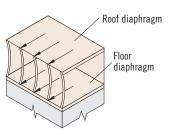
Wall is supported at top by roof diaphragm and at bottom by floor diaphragm.
