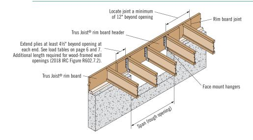
Support TII® joists from rim board header with face mount hangers only. For 1-ply header applications, reduce hanger capacities according to hanger manufacturer's recommendations.
